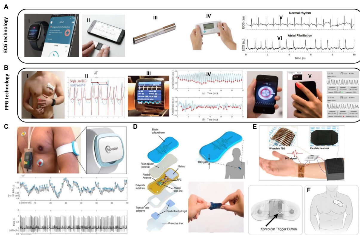
FIGURE 2 Wearable biosensors applications in cardiovascular care. (A) Examples of wearable tools used in clinical settings for ECG monitoring: (I) Fitbit-© Fitbit Inc., San Francisco, CA, United States, all rights reserved. (II) KardiaMobile-© all rights reserved (Mountainview, CA). (III) MyDiagnostick-© Applied Biomedical Systems BV, Maastricht, Netherlands, all rights reserved. (IV) Zenicor-ECG© Zenicor Medical Systems Ltd., London, United Kingdom, all rights reserved. (V) A sample of ECG graph for a healthy heart and, (VI) Afib ECG graph with irregular intervals. (B) Examples of wearable tools for PPG monitoring: (I) anatomical location of fibrichex patch on the chest-© Qompium, Hasselt, Belgium, all rights reserved. (II) Single lead ECG signal and fibrichex PPG signal. Reprinted from reference (25), licensed under CC BY 4.0. (III) Wristband of the Simband with LEDs for PPG and ECG. (IV) A sample 30 s clean PPG segment and corrupted PPG segment collected from Simband. Reprinted from reference (26), licensed under CC BY NC ND. (V) Smartphone camera-based PPG measurements of the pulse waveform. Reprinted from reference (27), licensed under CC BY 4.0. (C) Recorded PPG and ECG signals with the medical wearable attached to the left upper arm vs. ECG Holter (Everion, Biovotion AG, Switzerland). Reprinted from reference (28), licensed under CC BY. (D) Schematic illustration and image of a soft flexible cardiac sensor in a thin elastic enclosure consisting of the multiple polymeric, electronic, adhesive and hydrogel layers and data transfer to smartphone app (via NFC) for visualization of logged heart rate data and/or real-time ECG waveforms. Reprinted from reference (29), licensed under CC BY. (E) Schematic diagram of a flexible self-powered wearable ECG system. Reprinted from reference (30), Copyright © 2018 American Chemical Society. (F) Zio patch button and placement-© iRhythm Technologies, Inc., San Francisco, United States, all rights reserved.
