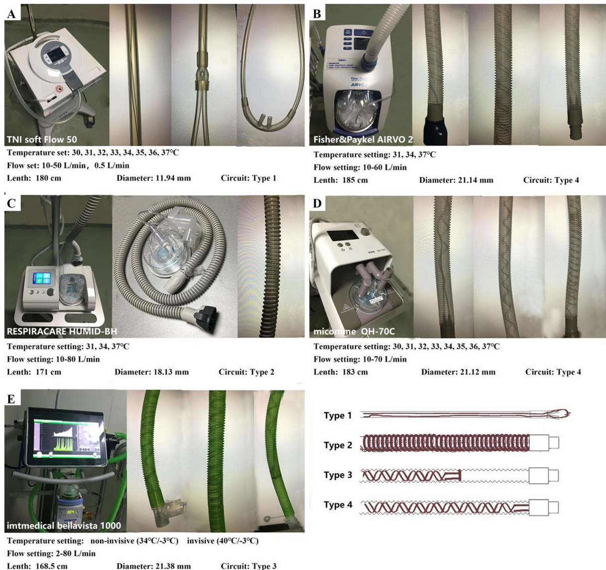
FIGURE 1 Settings of the HFNC devices and characteristics of the circuits. (A) TNI softFlow 50: The diameter of the circuit is smaller than other devices, and the heating wire is straight and runs through the whole circuit and the nasal cannulas (Type 1). (B,D) AIRVO 2 and OH-70C: the heating wire is arranged in a double helix structure in the whole circuit (Type 4). (C) HUMID-BH: The heating wire is wrapped in a spiral shape outside the circuit (Type 2). (E) Bellavista 1000 (MR850): the heating wire is arranged in a double helix structure in the circuit and located approximately 3/4 of the circuit near the humidifier (Type 3). Temperature sensors are installed both at the chamber outlet and the end of the heating circuit to provide feedback on the temperature and humidity output of MR850 in real time.
