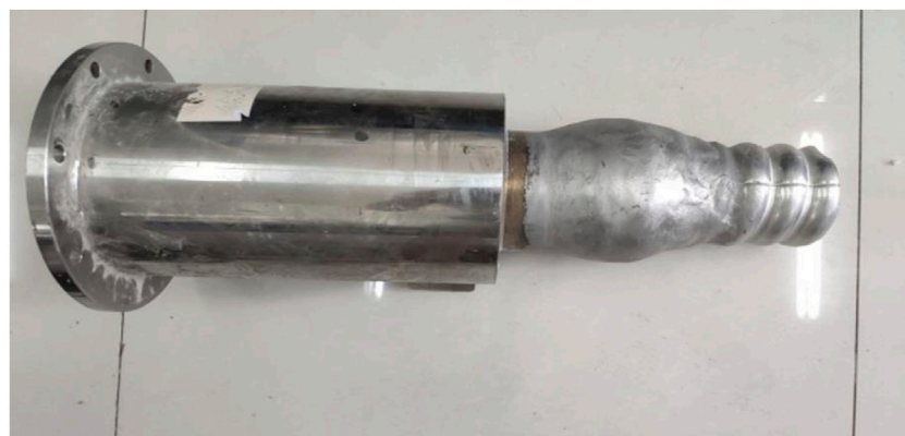
FIGURE 10 Cable terminal lead seal test sample.
