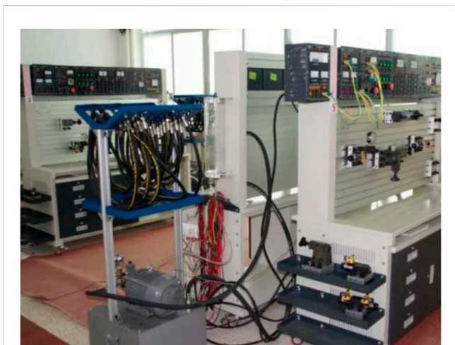
FIGURE 6 Hydraulic transmission test bench.
