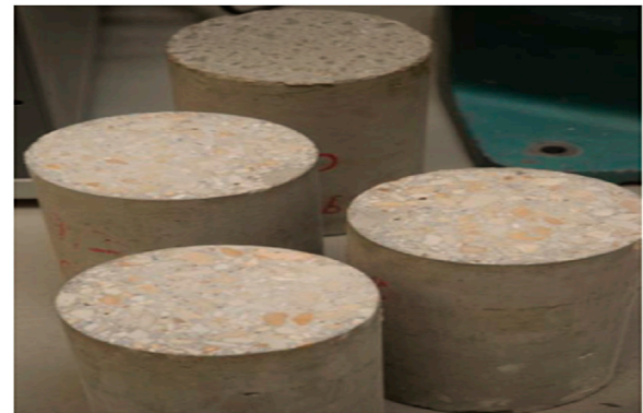
FIGURE 1 Some specimens prepared for buckling tests.
