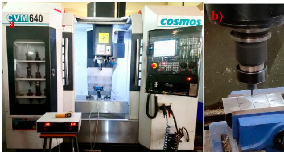
FIGURE 3 (A) Vertical Machining Center (VMC) (Alphonse et al., 2020a), (B) AZ31B is on the fixture and DLC-coated H13 tool steel is on the spindle head.
