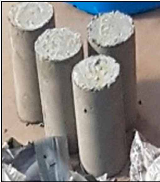
FIGURE 1 Prepared samples of cement with different ratios of waste ceramic aggregates.
