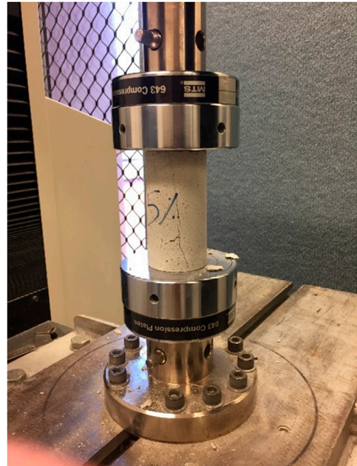
FIGURE 2 Photograph showing the sample under compressive loading conditions using the universal testing machine.
