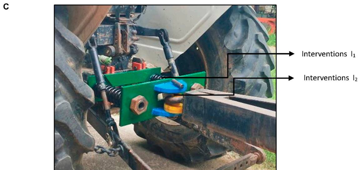
FIGURE 3 (A) CAD drawing of the spring-suspended tractor-trailer hitch (I 1 ); (B) PU bush (I 2 ); and (C) installed interventions I 1 + I 2 .
