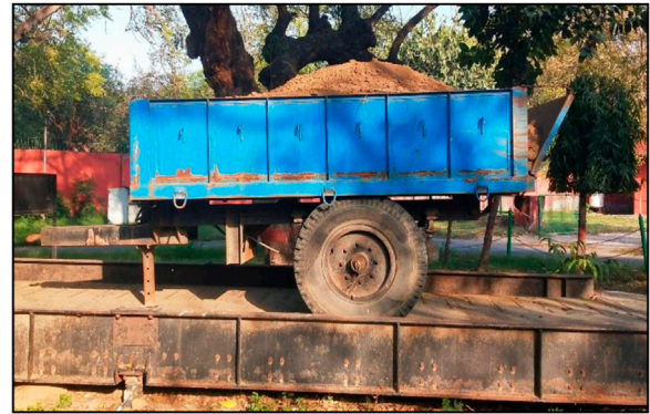
FIGURE 1 Fully loaded trailer on the weighing balance.
