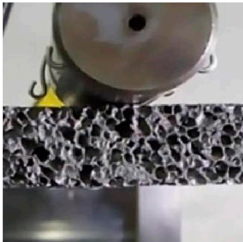
FIGURE 2 Carbon fiber-reinforced cold-cured resin–aluminum composite foam-core sandwich (Ashutosh et al., 2020).
