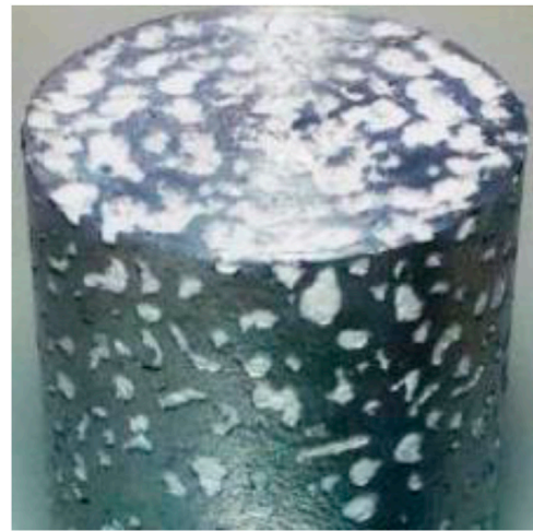
FIGURE 3 Expanded perlite–aluminum composite foam (Taherishargh et al., 2014).
