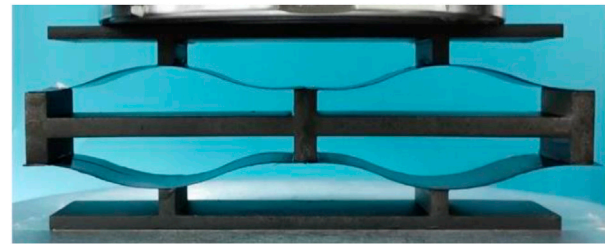
FIGURE 13 Continuous carbon fiber-reinforced polymer composite with a negative stiffness mechanical metamaterial (Chen et al., 2022).
