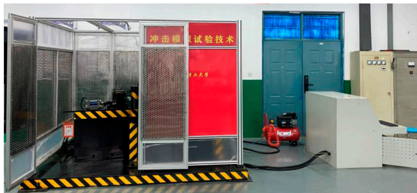
FIGURE 21 High-speed multi-layer target penetration simulation test system (Li, 2022).
