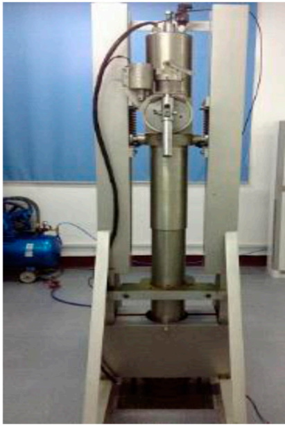
FIGURE 20 Single-impact testing apparatus (Man et al., 2014).
