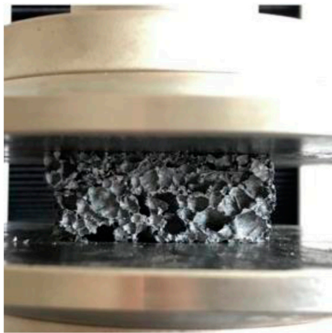
FIGURE 1 Aluminum–silicon carbide composite foam (Michał et al., 2022).
