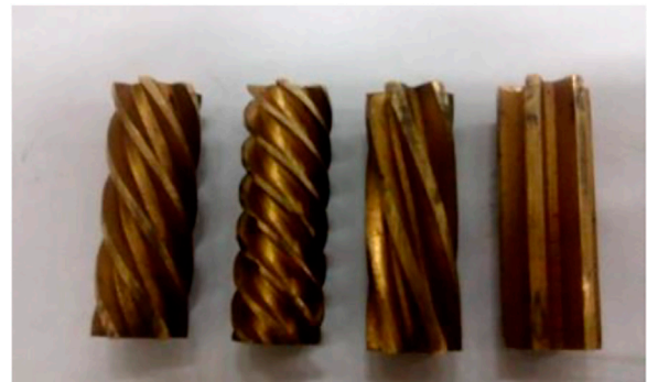
FIGURE 2 Swirl generators used in the experiment.
