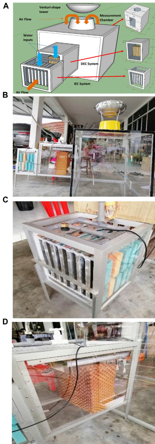
FIGURE 1 (A) Conceptual drawing of the proposed WIEC passive system with the indication of air flow and water input direction. (B) Corresponding assembled WIEC passive system with major components shown as (C) IEC component and (D) DEC component.
