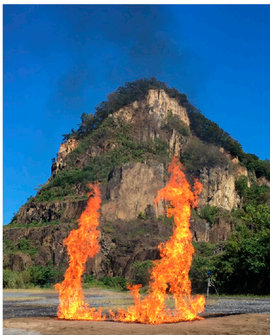
FIGURE 1 Figure 1A Fire whirls formed over an L-shaped line fire in an open-field experiment (Kuwana et al., 2022) Figure 1B (right) Type-I, II, III fire whirls (Kuwana et al., 2007).
