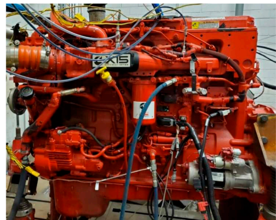
FIGURE 3 Cummins X15 engine platform installed in test cell.
