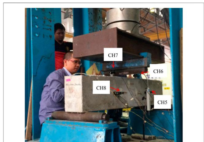
**FIGURE 6 |** Beam set up and set up of all instrumentations.
