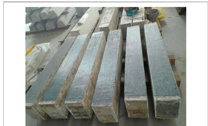
**FIGURE 4 |** The installed CFRP on the beam surface.
