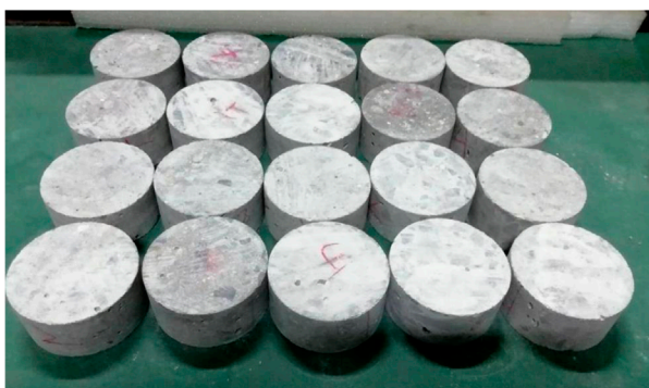
FIGURE 2 Partial processed concrete specimens.
