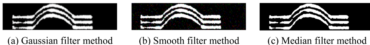
FIGURE 17 Filtering effect diagram. (A) Gaussian filter method. (B) Smooth filter method. (C) Median filter method.
