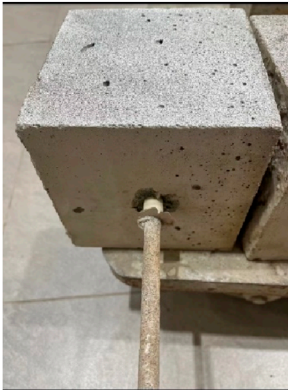
FIGURE 3 Center pull-out failure.
