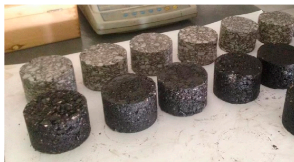
FIGURE 7 Bituminous samples prepared using superpave (grey) and marshall (black) mix design methods.
