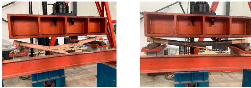
(a) Loading failure form of unreinforced members (b) Loading failure form of members after reinforcement failure
