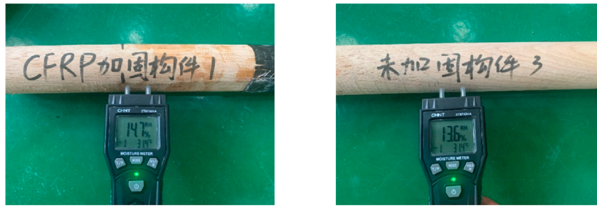
(a) Moisture content of reinforced members (b) moisture content of unreinforced members
