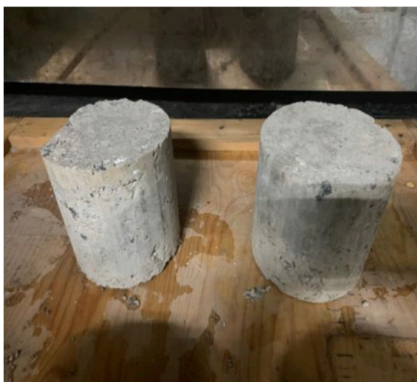
FIGURE 1 Cement-stabilized macadam specimen.
