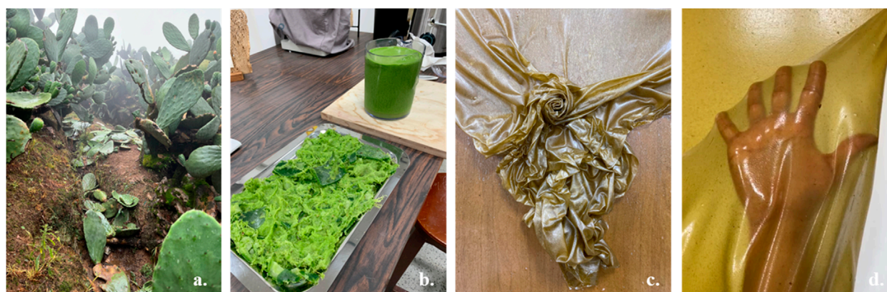
FIGURE 1 Biopolymer fabrication from nopal wastes: (A) Residues from leaves (cladodes) resulting from pruning, (B) Nopal mucilage extraction from cladodes and fibrous residues produced, (C) Biopolymer demolding and visual elastic properties demonstration, and (D) Flexible biopolymer with fabric-like characteristics.
