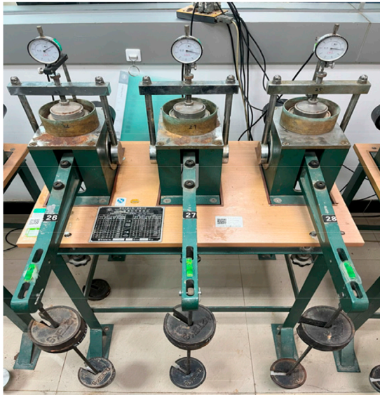
FIGURE 4 Standard consolidation experiment setup.
