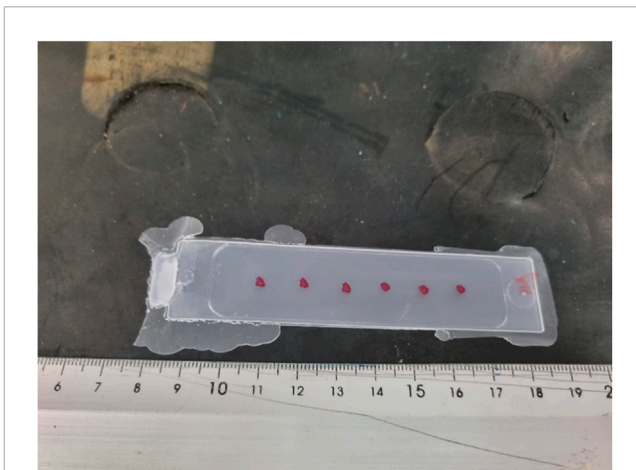
FIGURE 3 A photograph of a part fabricated by injection moulding using the operando equipment described in this manuscript. The red dots were added afterwards and mark the location of the six "windows" or sampling points.
