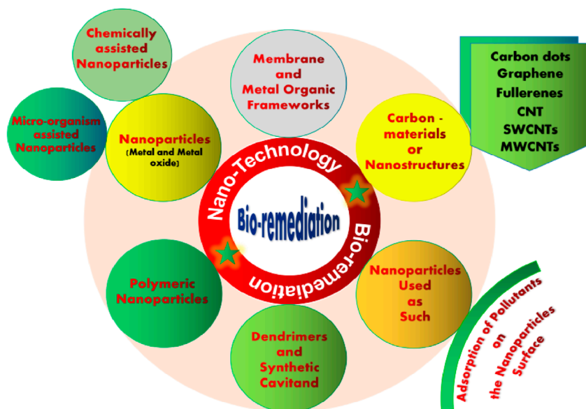
FIGURE 7 Microbial-assisted nanotechnology for bioremediation of wastewater. MOFs: Metal organic frameworks; MWCNTs: multi-walled carbon nanotubes; SWCNTs: Single-walled carbon nanotubes.
