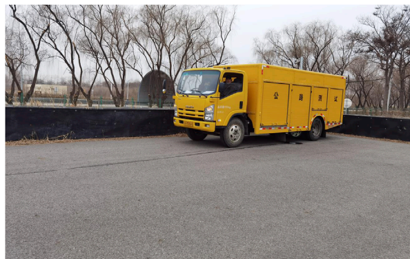
FIGURE 2 FC-2007 lateral force coefficient testing vehicle.
