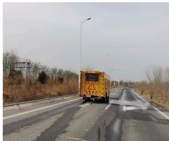
FIGURE 5 SFC testing process (different water film thicknesses).
