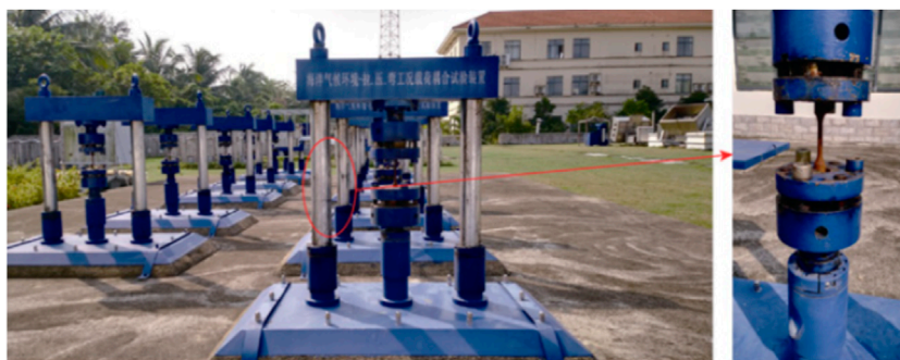
FIGURE 12 Coupling test platform of marine atmospheric environment and tensile/compression/bending load (Luo et al., 2021).
