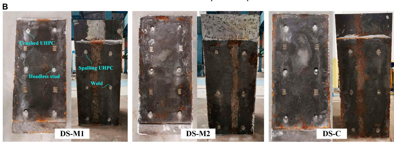
Inner surface of the UHPC slabs and steel plates
