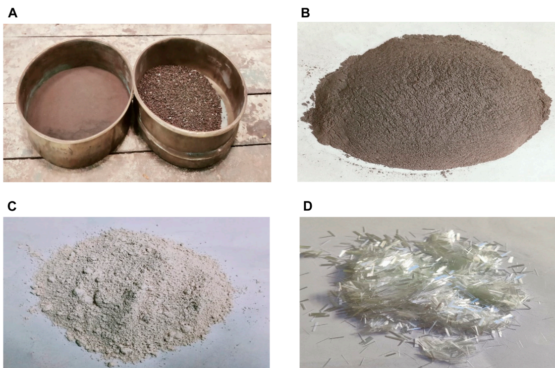
FIGURE 3 Raw materials for SCC: (A) raw BA, (B) sieved BA, (C) MK, and (D) GF.
