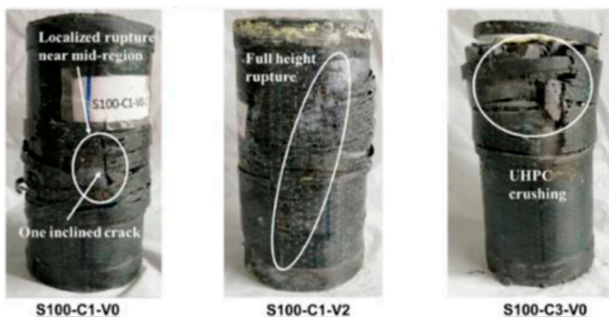
FIGURE 1 Carbon FRP constrained specimen failure morphology (Liao et al., 2021).
