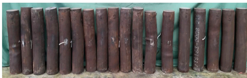
FIGURE 4 Shape of the test short columns after failure.
