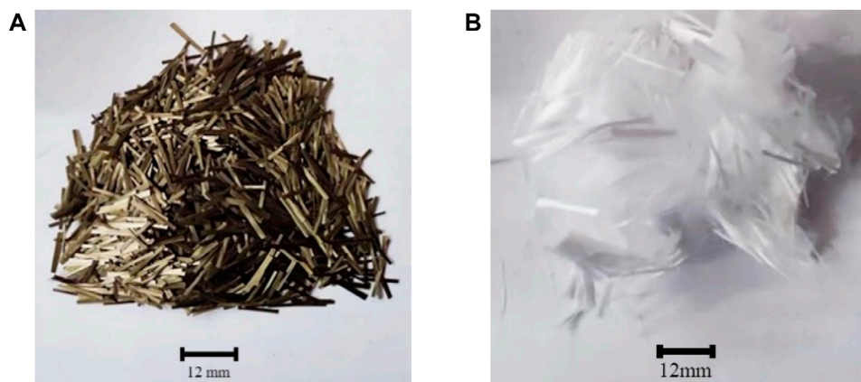
FIGURE 1 Fibers: (A) Short-cut basalt fiber; (B) Short-cut polypropylene fiber.
