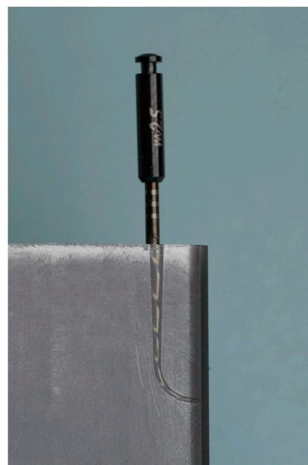
FIGURE 3 Artificial stainless-steel canal for dynamic cyclic fatigue test.
