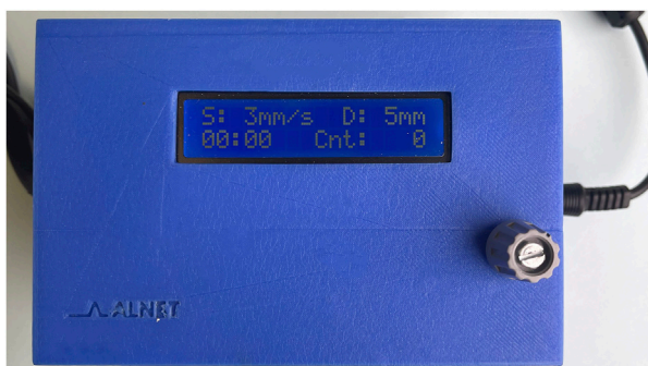
FIGURE 2 Dynamic cyclic fatigue test's device computer module.
