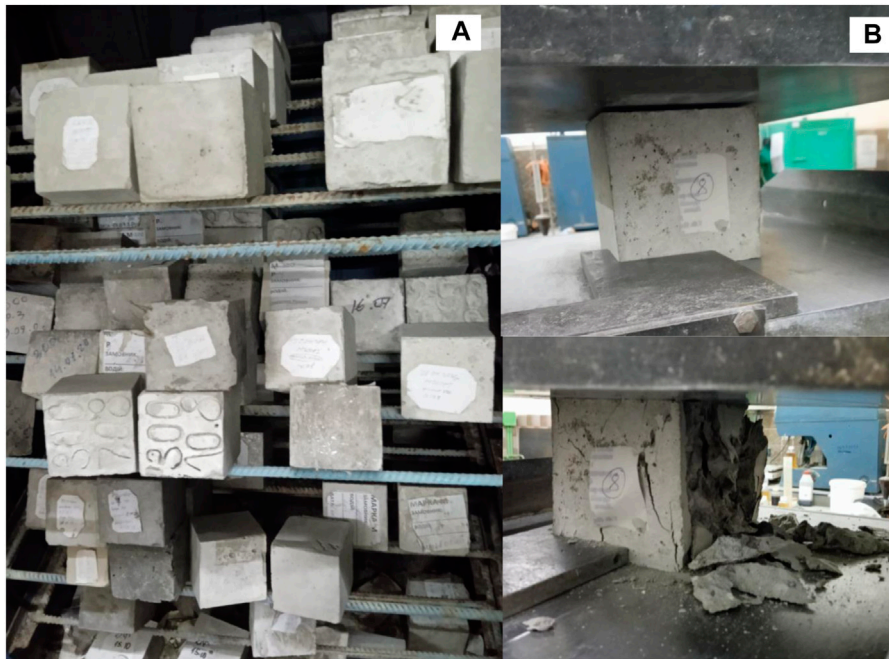
FIGURE 4 Concrete samples with LKD and their testing: (A) normal hardening chamber; (B) sample before and after determination of compressive strength.
