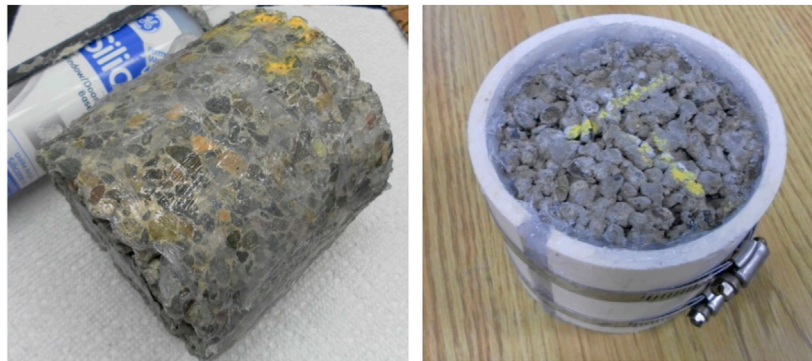
FIGURE 3 Pictures of water permeability testing preparation.
