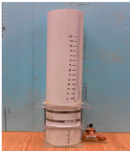
FIGURE 4 The test equipment for water permeability.
