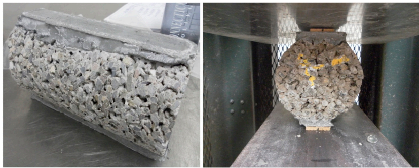
FIGURE 2 Splitting tensile strength test process.
