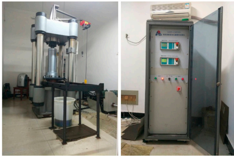
FIGURE 4 RLW-2000 Microcomputer controlled triaxial creep testing machine.
