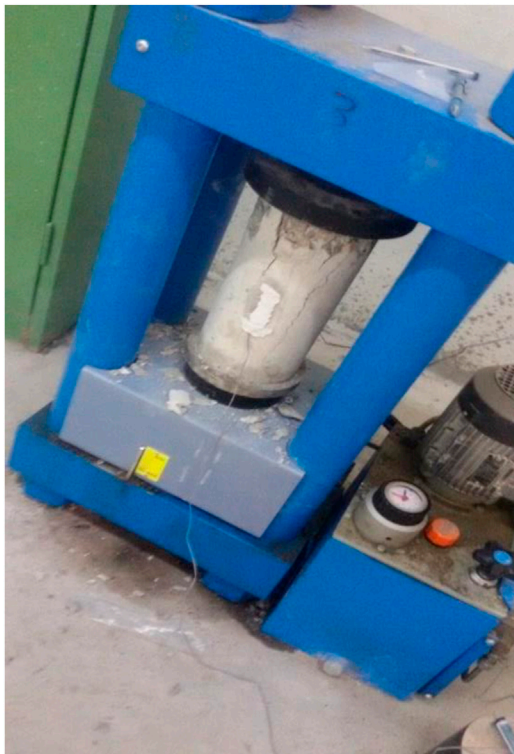
FIGURE 8 A sample of modulus of elasticity test.
