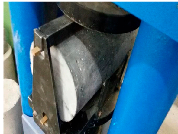
FIGURE 6 A sample of the tensile splitting test.
