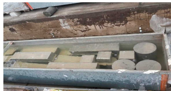
FIGURE 3 Specimens being cured in wet conditions.
