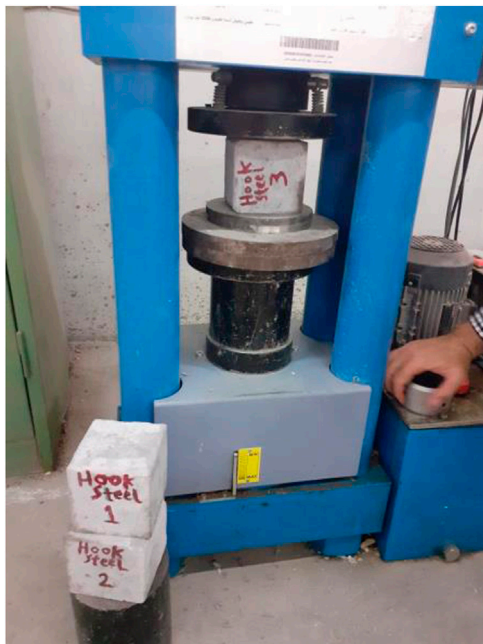
FIGURE 5 A sample of compressive strength test.
