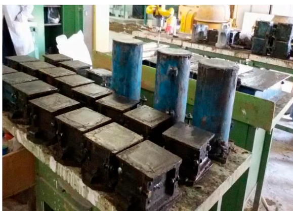
FIGURE 2 Cast specimens in cube and cylinder molds.
