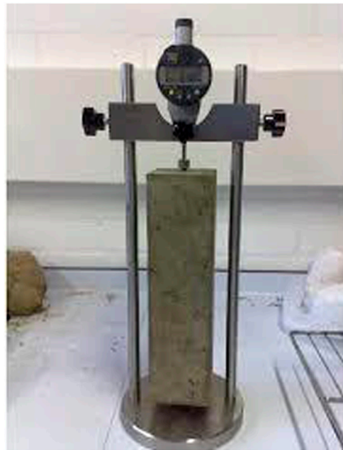
FIGURE 9 Drying shrinkage test.
