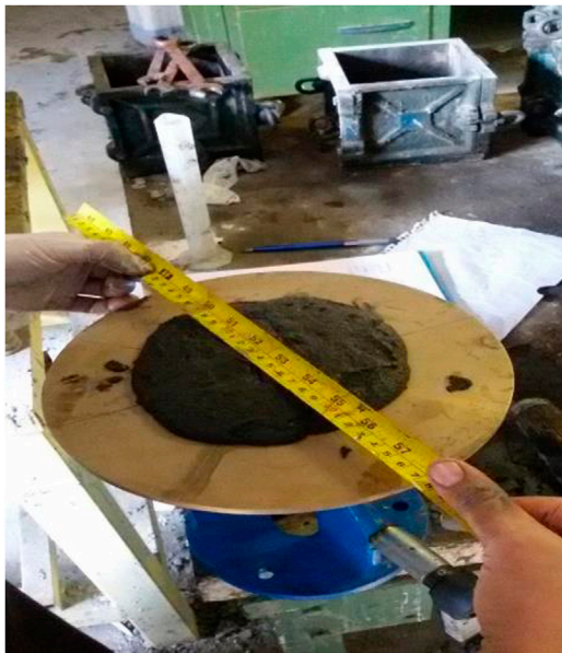
FIGURE 4 A sample of the flow table test.
