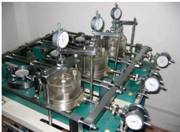
FIGURE 4 Physical picture of the improved direct shear creep apparatus.
