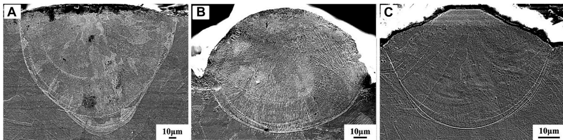
FIGURE 7 The effect of LED on microstructure: (A) P = 160 W, V = 300 mm/s, LED = 272 J/mm 3 , (B) P = 100 W, V = 200 mm/s, LED = 255 J/mm 3 , (C) P = 130 W, V = 900 mm/s, LED = 74 J/mm 3 .
