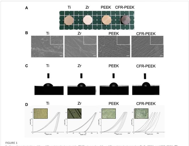
Surface characterization of four different implant materials. (A) Photographs of four different implant samples: Ti, Zr, PEEK, and CFR-PEEK. (B) FE-SEM images of Ti, Zr, PEEK, and CFR-PEEK samples under low and high magnifications (2000x, bar = 5  $\mu$ M; 5,000x, bar = 2  $\mu$ M). (C) The contact angle of different samples. (D) The load-displacement curves for different samples, where the upper-left image shows an optical microscope image (1,000x, bar = 10  $\mu$ M) of the punctured area.
