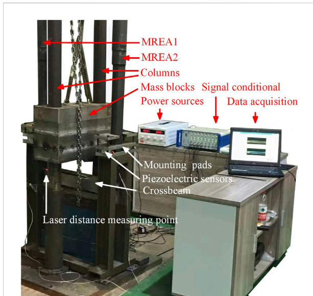
FIGURE 5 Experiments based on the drop test bench.
