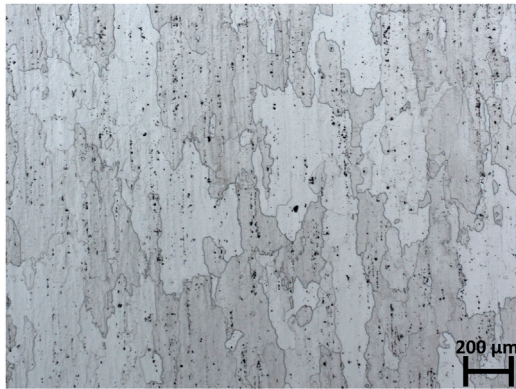
FIGURE 2 | Optical micrograph of the Al 7075 T651 plate. The representative average grain size is 135 \pm 70 \mu\text{m} estimated by line intercept method.
