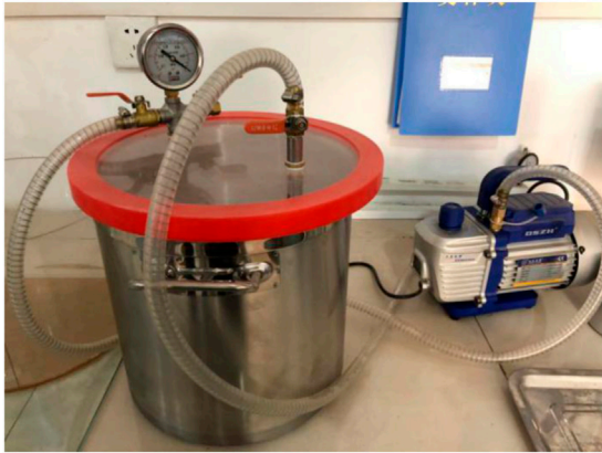
FIGURE 2 | Negative pressure strengthening equipment.
