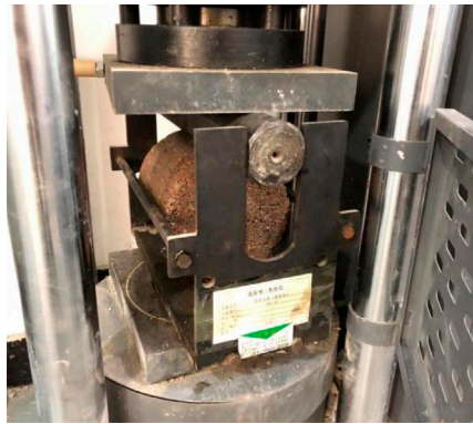
FIGURE 14 | Law of indirect tensile strength.
