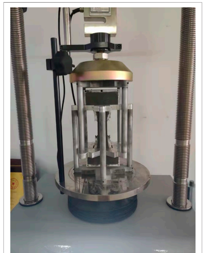
FIGURE 5 | Direct tensile test of the dog-bone CPB specimen.
