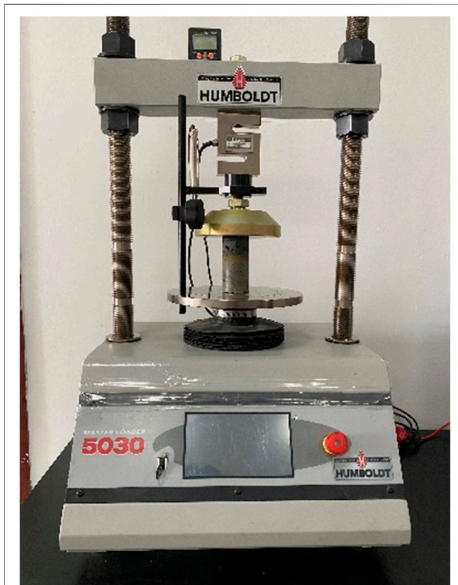
FIGURE 4 | Unconfined compressive test of the cylindrical CPB specimen.
