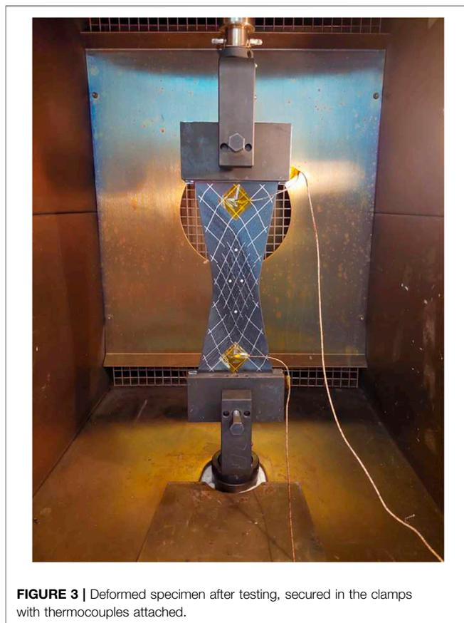
placed between the clamps in the preheated climate chamber. The clamps were tightened by hand with medium force to prevent excessive squeeze out of the tape material. **Figure 3** shows a clamped specimen (after testing).
