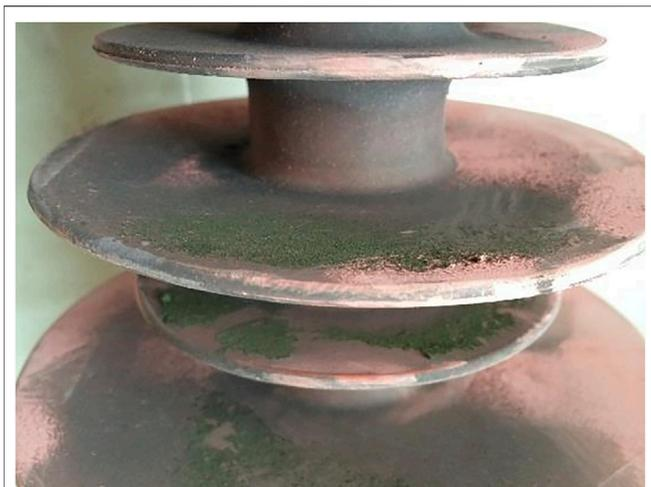
**FIGURE 2** | Morphology of fungi-fouled insulator.
