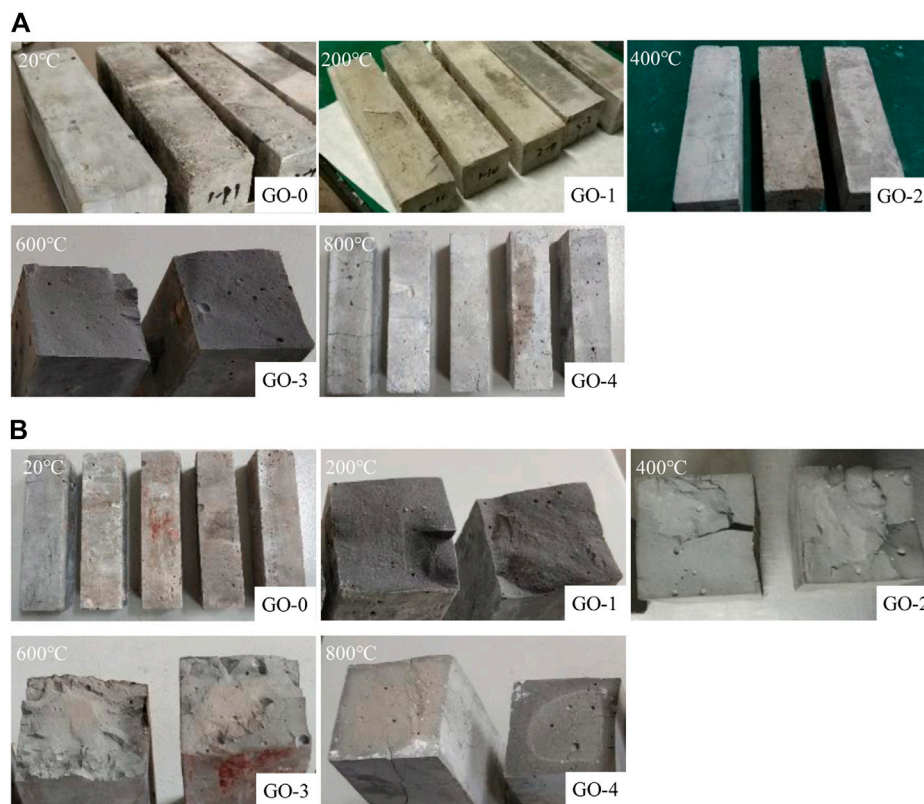
FIGURE 1 | Surface topographies of GORC after 28-day curing period exposure to different high temperatures (A) and their fractured counterparts (B) . Note: the specimens are observed to spontaneously break at 800°C.
