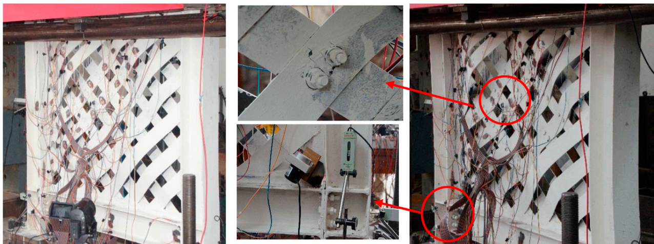
FIGURE 7 The IWS-SPSW specimen failure phenomenon.
