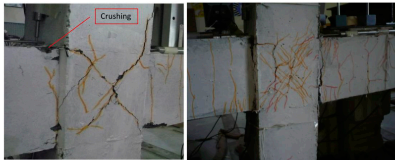
FIGURE 5 (A) Crushing of concrete in RC specimen (B) Crack patterns in SHCC enhanced specimen.
