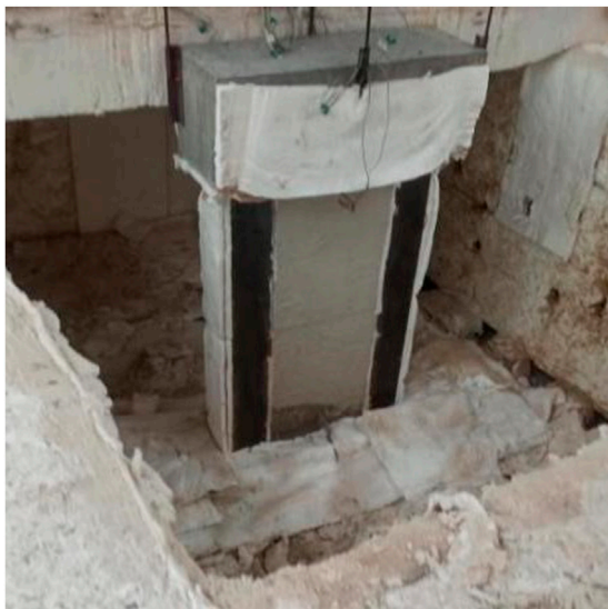
FIGURE 5 Fire protection treatment of specimens.
