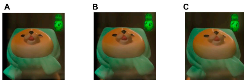
FIGURE 9 | Reconstructed images in the holographic near-eye display obtained from (A) left -7^\circ direction, (B) center 0^\circ direction and (C) right 7^\circ direction.
